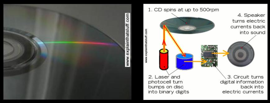
So the real energy transformation includes lasers. Here it is: electrical mechanical (disc spins) mechanical (laser) mechanical (sound)
