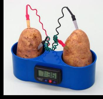
The potato is used as the battery to make the clock run. A battery is a type of electrochemical cell that converts chemical energy into electrical energy.
