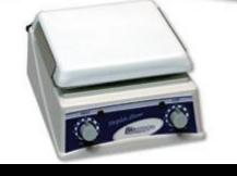
A hot plate transforms electrical energy into heat (thermal energy). This energy is then transferred to the object on it (a beaker usually) by conduction.
